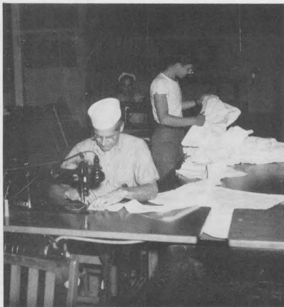
THE SAIL-MAKERS' SHOP. Grizzled Bosun's Mate Herrick of the 83rd Battalion is shown engaged in the fabrication of certain necessary canvas gear. Not only sails, but seat cushions, awnings, canopies and bags are turned out here. The art of the sailor's palm and needle survived the advent of steam.
